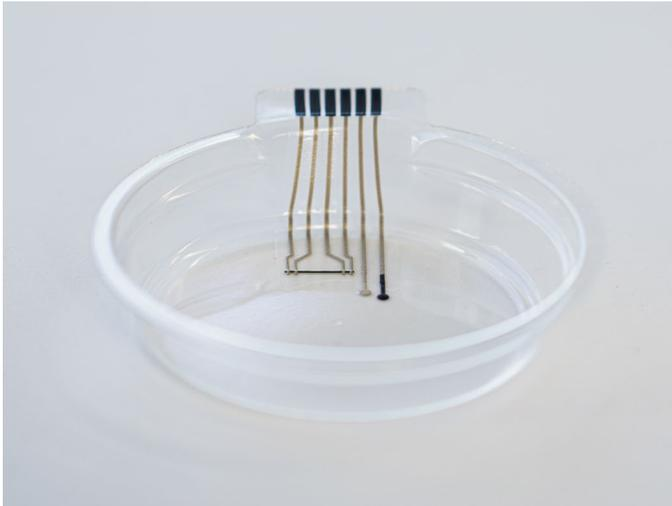
**Caption:** Intelligent sensors are printed on films and subsequently thermoformed to create smart petri dishes.
